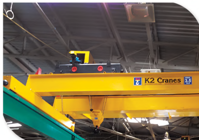
DOUBLE GIRDER EOT CRANE CAPACITY: Up to 150 ton
