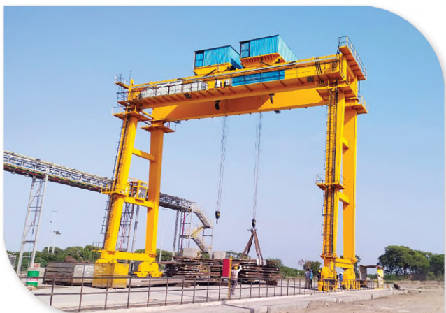
GANTRY CRANE CAPACITY: Up to 300 ton
