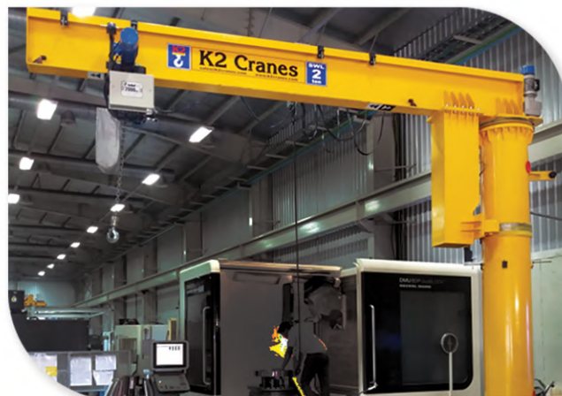
JIB CRANE CAPACITY: Up to 5 ton
